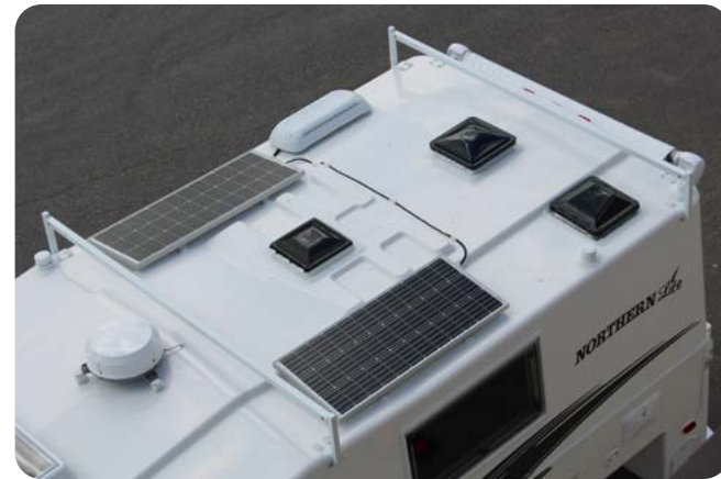
Boat Rack and Dual Solar Panels
