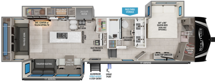
310GK U W 1 12,100 HITCH 1 2,350 GVWR 15,000 LENGTH 2 34' 4" HEIGHT 3 13' 5" CAPACITY 81 106 53
