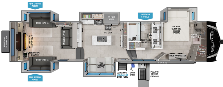
376RD U W 1 15,180 HITCH 1 3,050 GVWR 18,000 LENGTH 2 42' 5" HEIGHT 3 13' 5" CAPACITY 81 106 53
