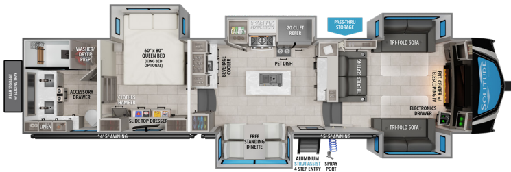
382WB U W 1 14,866 HITCH 1 3,052 GVWR 18,000 LENGTH 2 41' 4" HEIGHT 3 13' 5" CAPACITY 81 106 53
