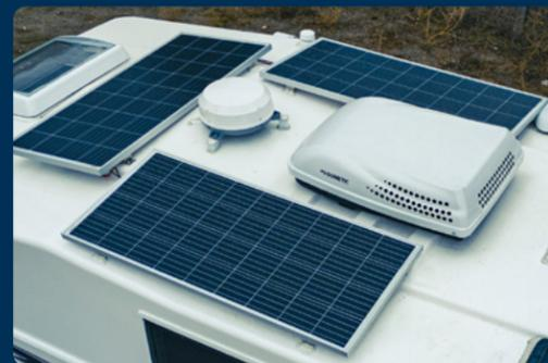
600 Watts of Solar Panels on ALL models
