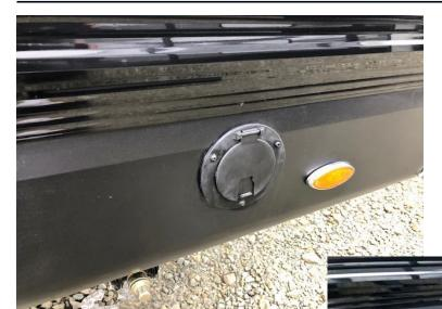
Behind this door latch is a 2" receiver bolted to the frame and lagged to the floor.
