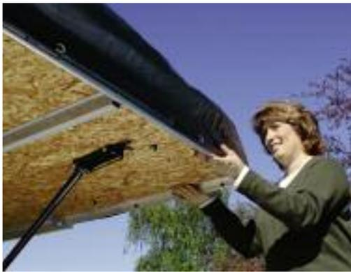
"Weyerhaeuser agrees with Fleetwood's practice of not coating the exposed bottom surface of the Structurwood® panels used in their trailers. In our opinion, moisture from occupancy load, or from other internal or external sources may become trapped in the Structurwood® substrate if it is coated on the underside with a system that impairs the ability of the substrate to dry thoroughly. Trapped moisture, over time, may cause premature decay or rot." Weyerhaeuser
