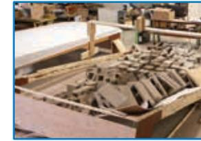
4. **Durable floors** feature 5/8-inch tongue-and-groove plywood (n/a on 7-foot Jay Flight SLX) on 2-inch x 3-inch wooden joists, wrapped with a protective moisture barrier to keep the elements at bay
