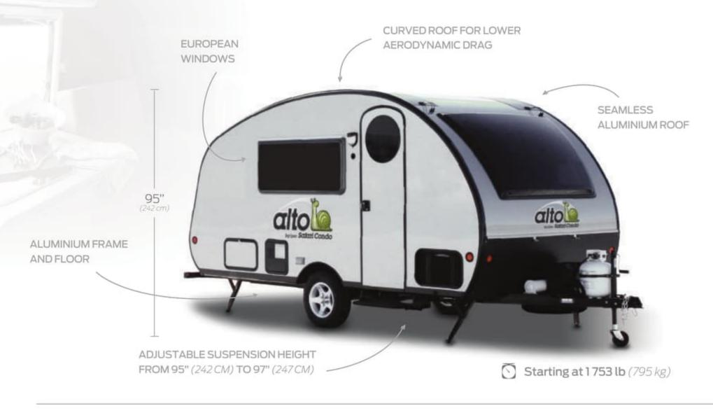
european style Alta Imported from Europe, the double glazed panoramic acrylic windows of the F series provide both lightweight and superior insulation. The windows include a built-in combination blind/screen system. This type of window provides such a large opening that one almost forgets being inside. The front dinette, with its huge curved window, can be used even while the rear bed is deployed. In addition, by moving the table, it is possible to create a four seat dining area.
