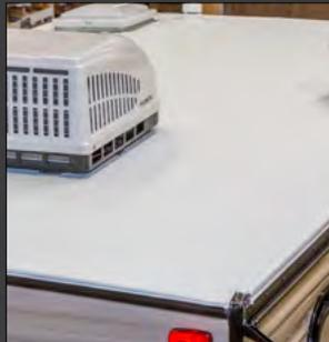
Seamless Roofing Membrane with Heat Reflectivity
