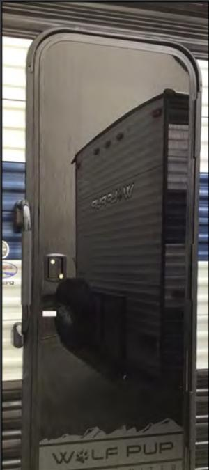
Real Blackout Glass, Safety Slam, Friction Hinge Entry Door with Window and Shade Prep
