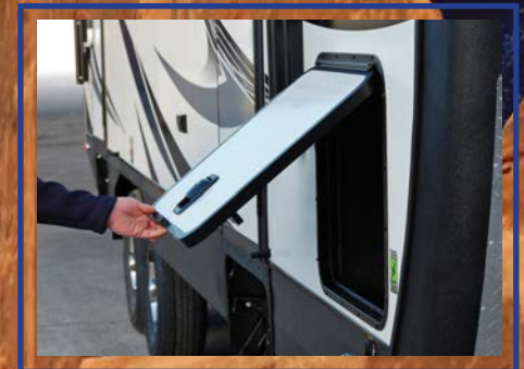
1" Thick Thermal Insulated Luggage Door Compartments
