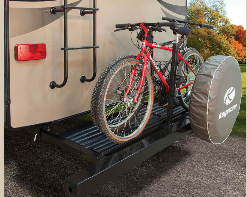
Another Cougar first: The rear storage rack provides a quick slide-away storage alternative.
