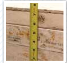
7" HEADER BEAM VS. 2" X 6" LUMBER
