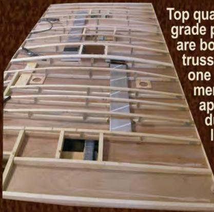
Top quality exterior grade plywood panels are bonded to the trusses and a thick one piece roofing membrane is then applied for a durable, long lasting seal to protect you and your coach from the elements.
