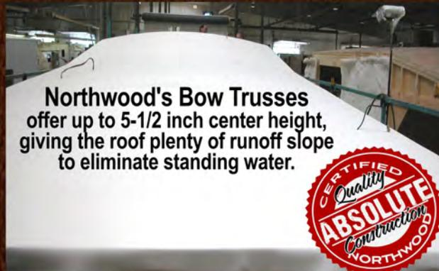
Northwood's Bow Trusses offer up to 5-1/2 inch center height, giving the roof plenty of runoff slope to eliminate standing water.
