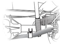
**HEAVY-DUTY FRONT & REAR STABILIZER BAR** A larger bar and polyurethane bushings, instead of rubber, transfer power faster for extra support, more stability and easier handling
