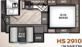
Ext. Length (with Ladder): 19'3" Ext. Width: 8'2" Floor Length: 10' Wheel Well Width: 48"
