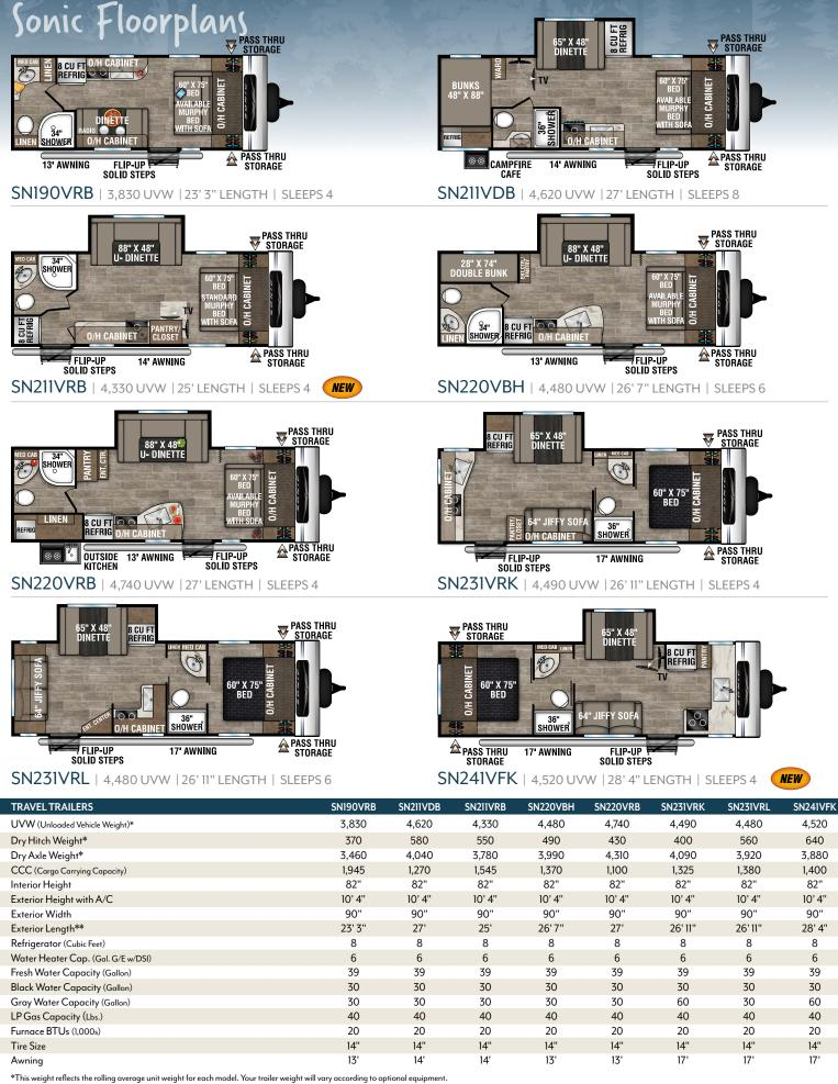
\*\*Exterior length is measured from rear of bumper to leading edge of coupler.
